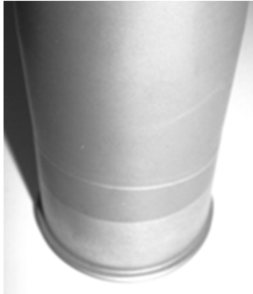
Figure 1.—ASC-E2 heater head: The SN18 heater head test article after completion of permeability testing and removal of the permeometer flange hardware.
